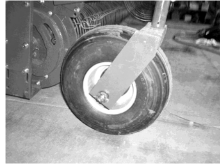
Pickup head tire Tire size-18 x 9.5-8 Maintain 24 lbs. (165 kPa) pressure
