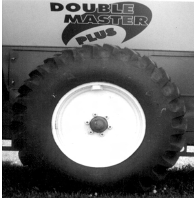
Tire size-18.4 x 30 Maintain 20 lbs. (140 kPa) pressure
